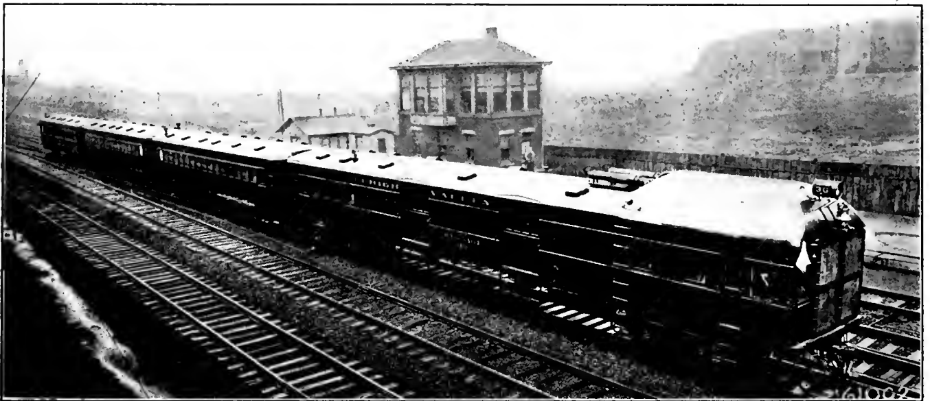
Fig. 1. Lehigh Valley Railroad Gas-Electric Train Consisting of Brill-Westinghouse Double Unit Motor Car and Trailers
